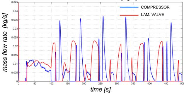
The thermodynamic system behaves as an open loop subsystem, under the following exogenous inputs to the model, which, together with the model output, allow closing the vehicle HVAC control loop and completing the set of influencing quantities:
