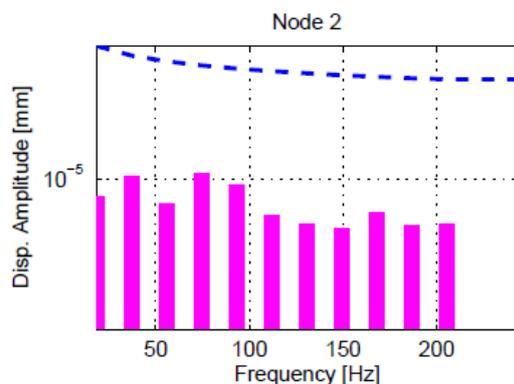
**MECHDYN™** result plots: comparison of vibration harmonics amplitude at a structure node with API 618 limits
