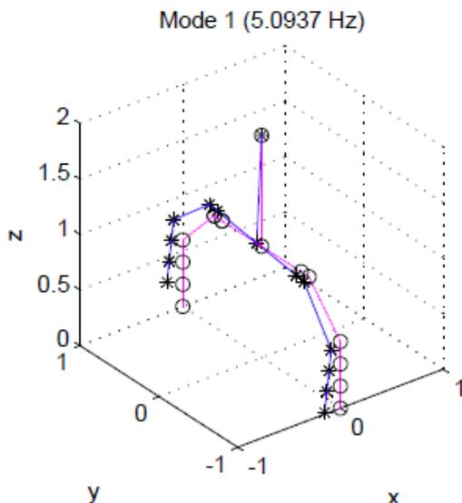
**MECHDYN™** result plots: undeformed structure (magenta) and vibrating modes (blue)
