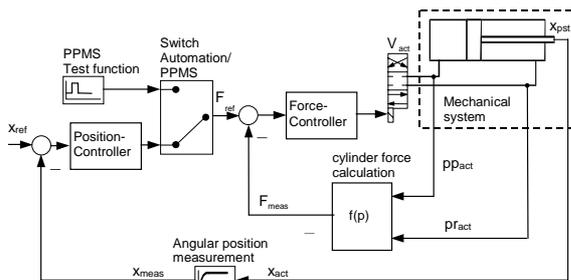
Fig. 3: Electric control of the hydraulic looper system
