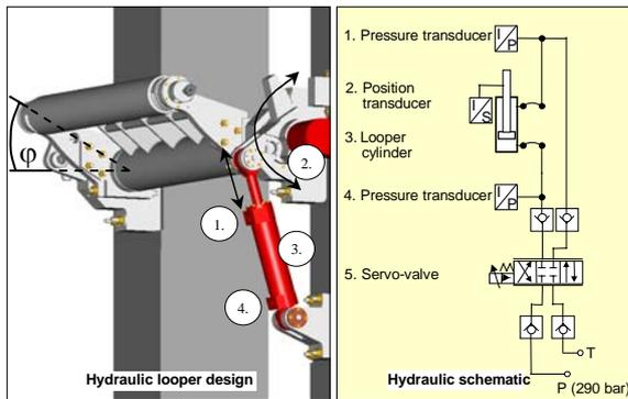
Fig. 2: Design of the hydraulic looper
