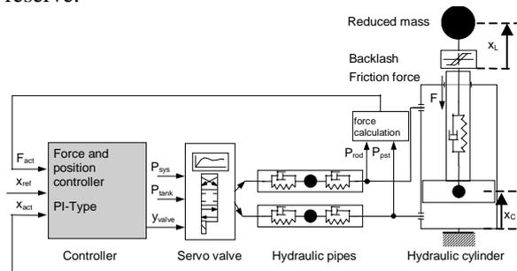
Fig. 4: Modelling of the hydraulic system
