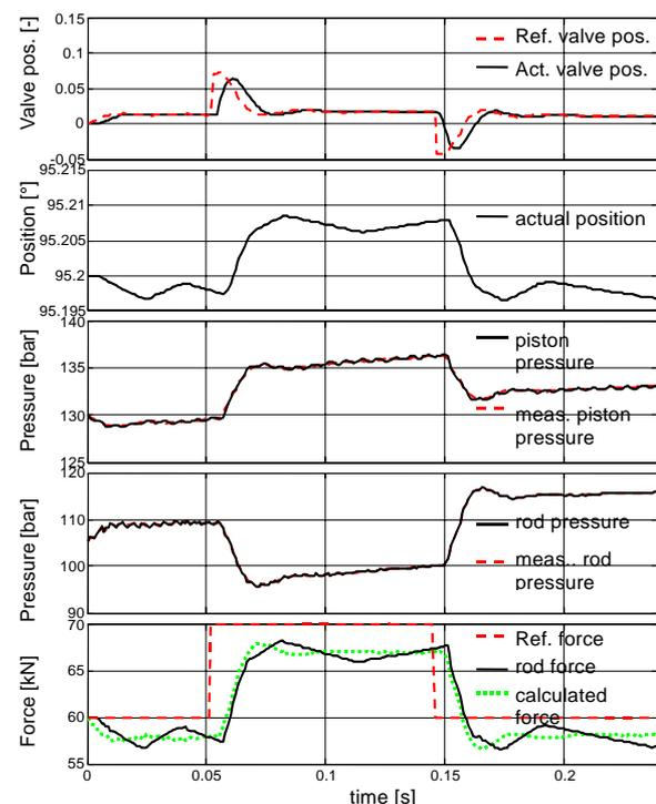
Fig. 6: Inner leak of  $10^{-6} \text{m}^2$  in hydraulic cylinder between piston and cylinder wall
