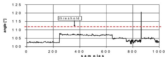
Fig. 7: Trend of the angle at top position of the looper
