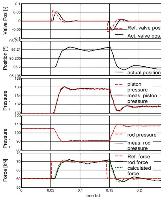
Fig. 5: Step response in force control: normal operation
