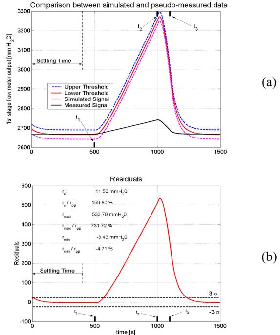
Fig. VI. Comparison between Pseudo-Measured and BB simulated signals of a testing set of BB model M1STMFR used with faulty condition 1STCBLEAK - fault starts developing in  $t_1$ ; fault stops developing in  $t_2$ ; fault ends in  $t_3$ .
