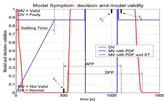
Fig. VII. Symptom obtained on the testing set of model M1STMFR used with faulty condition 1STCBLEAK - fault starts developing in  $t_1$ ; fault stops developing in  $t_2$ ; fault ends in  $t_3$ . AFP: Actual Fault Period. DFP: Detected Fault Period.
