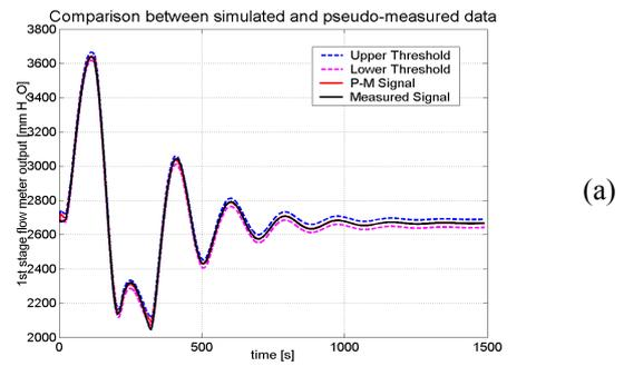
Fig. IV. Comparison between the Pseudo-Measured (P-M) and the simulated output signals with the training set of BB model M1STMFR (flow rate measurement is expressed in mmH<sub>2</sub>O).
