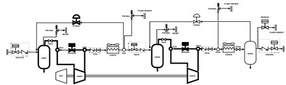
Fig. III. Simplified PFD of a typical gas compression train for a large pipeline booster station.
