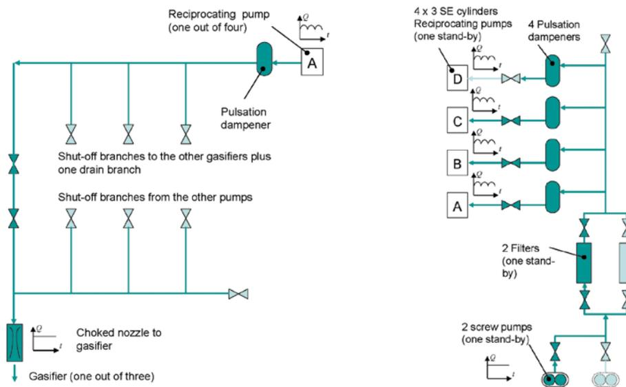
Figure 1. Scheme of the pumping plant following one of the possible suction side (right) and discharge side (left) configurations.
