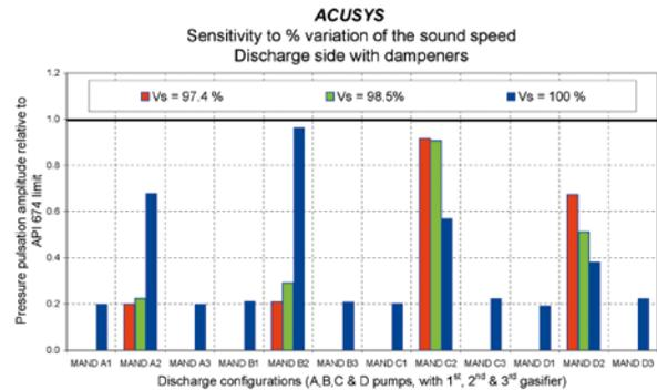
**Figure 6. Discharge piping: sensitivity analysis of the amplitude of the critical harmonic to the speed of sound 'Vs' in the fluid, expressed as ratio to the nominal design value (100%). In all cases the critical harmonic is 10 Hz.**
