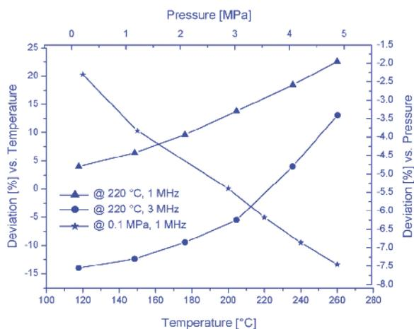
Figure 3. Variation of the sound speed in the process fluid (TAR), as a function of temperature (at constant pressure) or pressure (at constant temperature). The variations are expressed as a percentage of the reference value at the pumps discharge conditions (temperature 220 °C and pressure 4.2 MPa).
