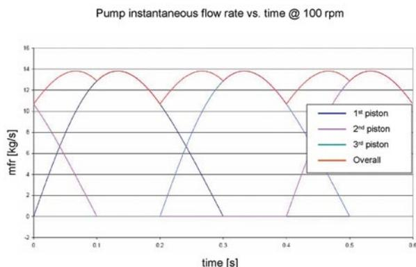
**Figure 2. Instantaneous mass flowrate vs. time by each piston and by a single whole pump (upper envelope) of the TAR pumping plant.**
