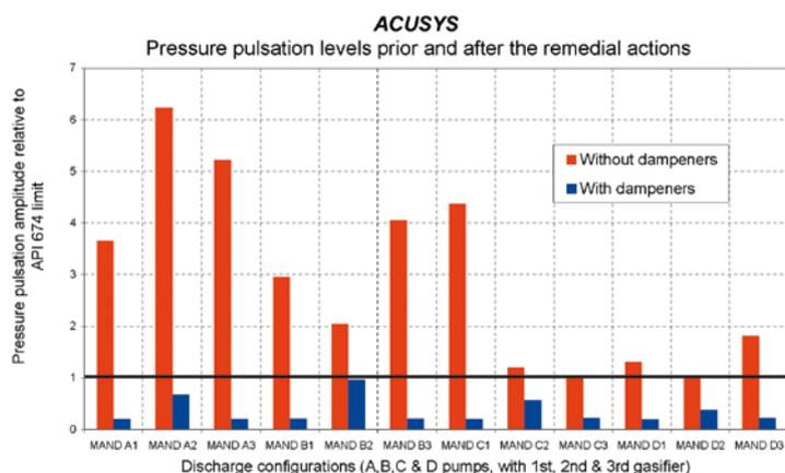
Figure 5. Discharge piping: reduction of the amplitude of the critical harmonic of the generated pressure pulsation obtained by the pulsation dampeners (blue columns), compared with the pulsations occurring prior to the plant modification (red columns) for each of the 12 discharge piping configurations. The values are expressed as ratio to the limit calculated according to API 674-sec.3.6<sup>1</sup>. In all cases the critical harmonic is 10 Hz.
