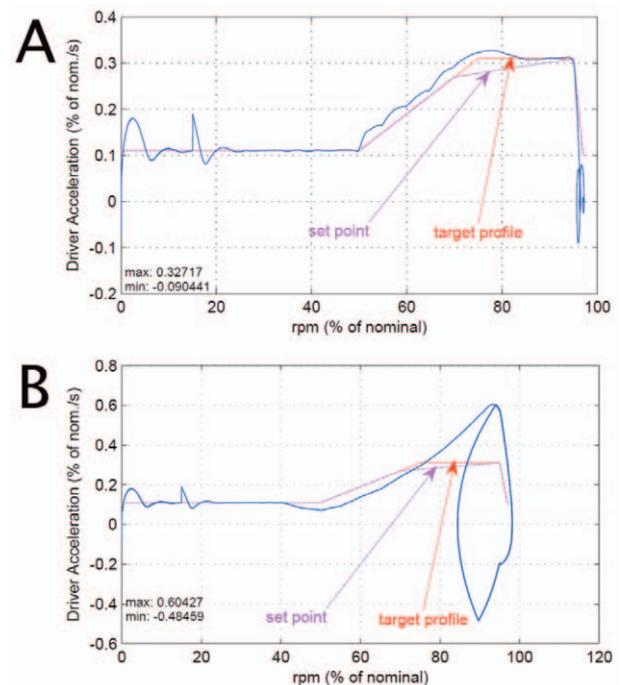
**Figure 5.** Case study two: driver acceleration versus speed during normal start up from depressurised conditions, from pressure below (A) and above (B) the instability starting pressure threshold, identified by DSS.
