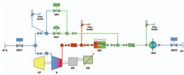
**Figure 4.** Case study two: simplified depiction of the modelled NGL extraction and liquefaction compressor.
