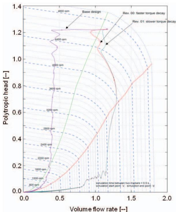
**Figure 3.** Case study one: compressor operating point (normalised units). As built, without hot bypass (magenta); as made after DSS, with hot bypass under the fastest (red) or slowest (black) driver torque decay rate.
