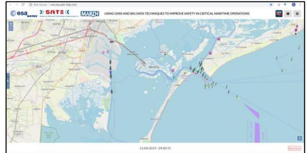
Vessels' real-time AIS data can be checked against the compatible preferred routes and generate alerts in case of deviation from the expected behaviour (either due to routes differences in position or timing/speed). This may allow *automatizing* (i.e. improve the efficiency of) the maritime surveillance operations highlighting to the operators those situations that require attention.
